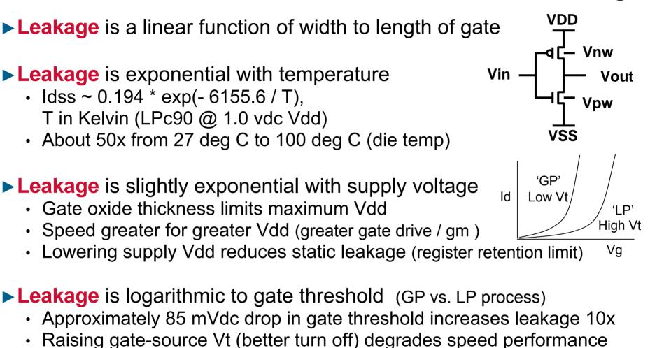
Process can be set to higher speed performance or lower leakage
